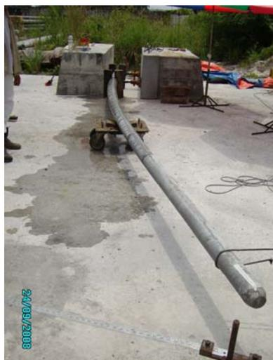
**Pole After Bending Test**
