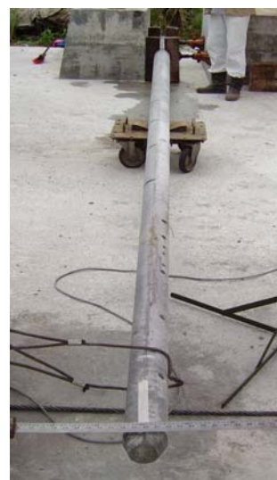
Pole After Bending Test (Back to original position)
