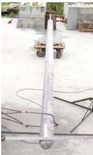
**Pole During Bending Test**
